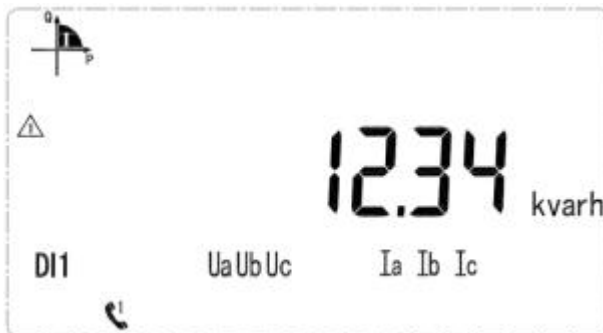
Current forward reactive energy 12.34kWh
